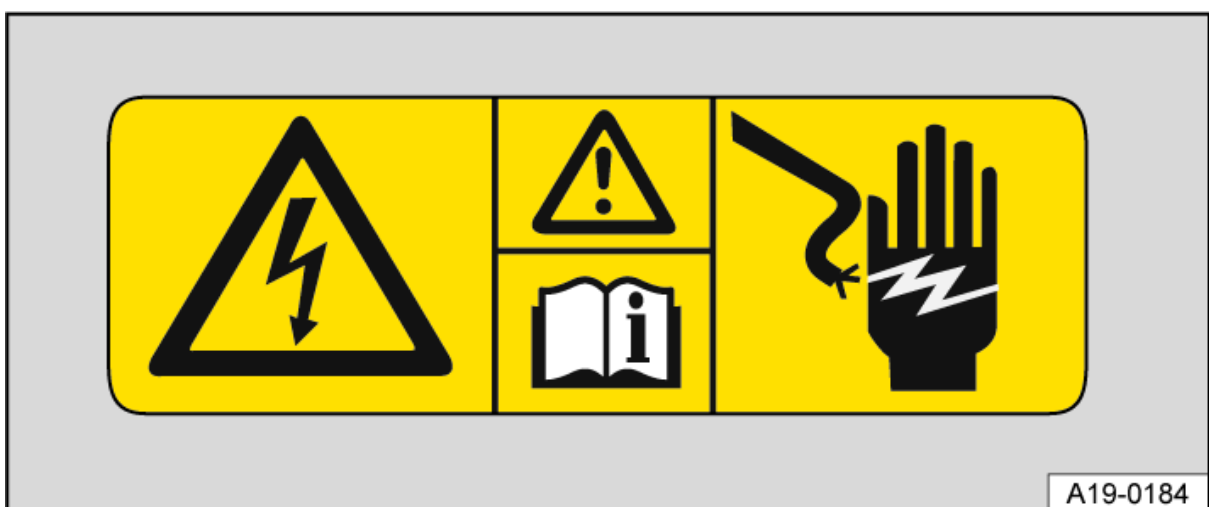
Fig. 2 Warning sign for high-voltage components.
