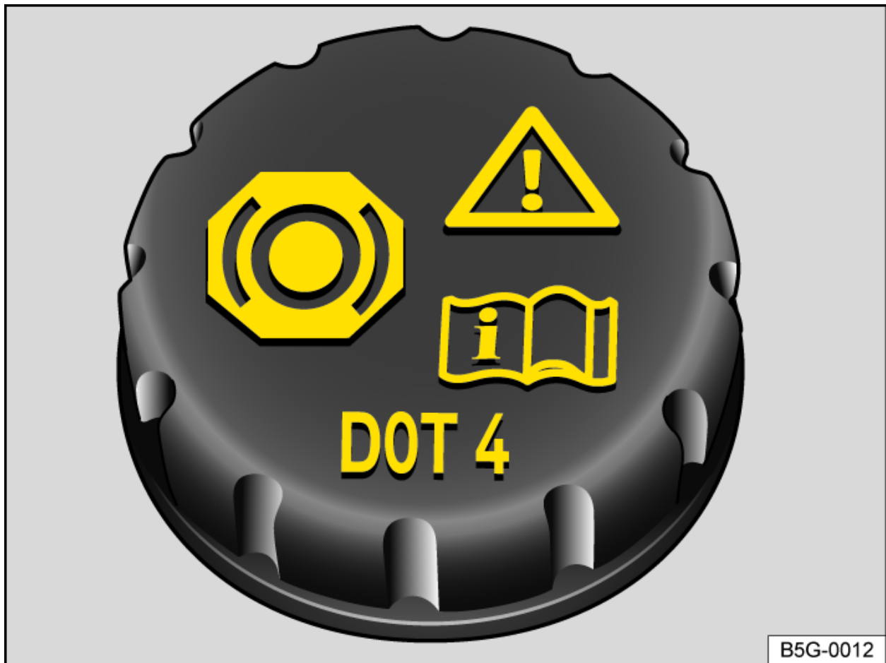
Fig. 1 In the front compartment: cap of the brake fluid reservoir.
