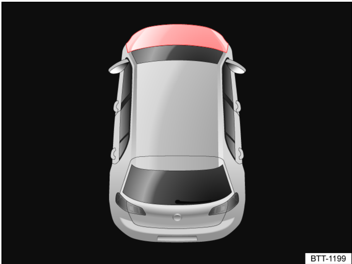
Fig. 1 On the instrument cluster display: the bonnet is open or not closed properly (illustration).
