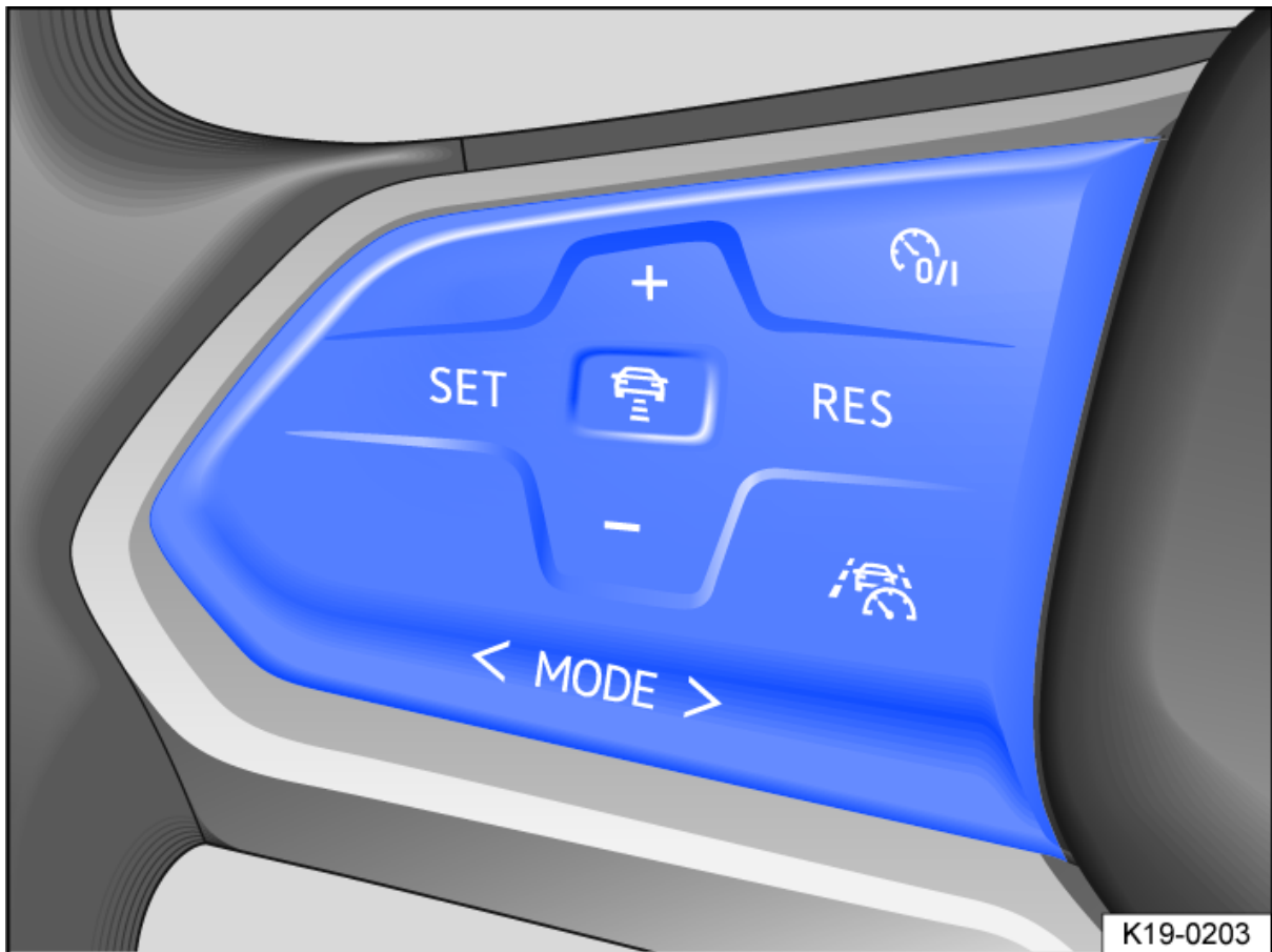
Fig. 1 Left-hand side of the multifunction steering wheel: buttons for operating Travel Assist.
