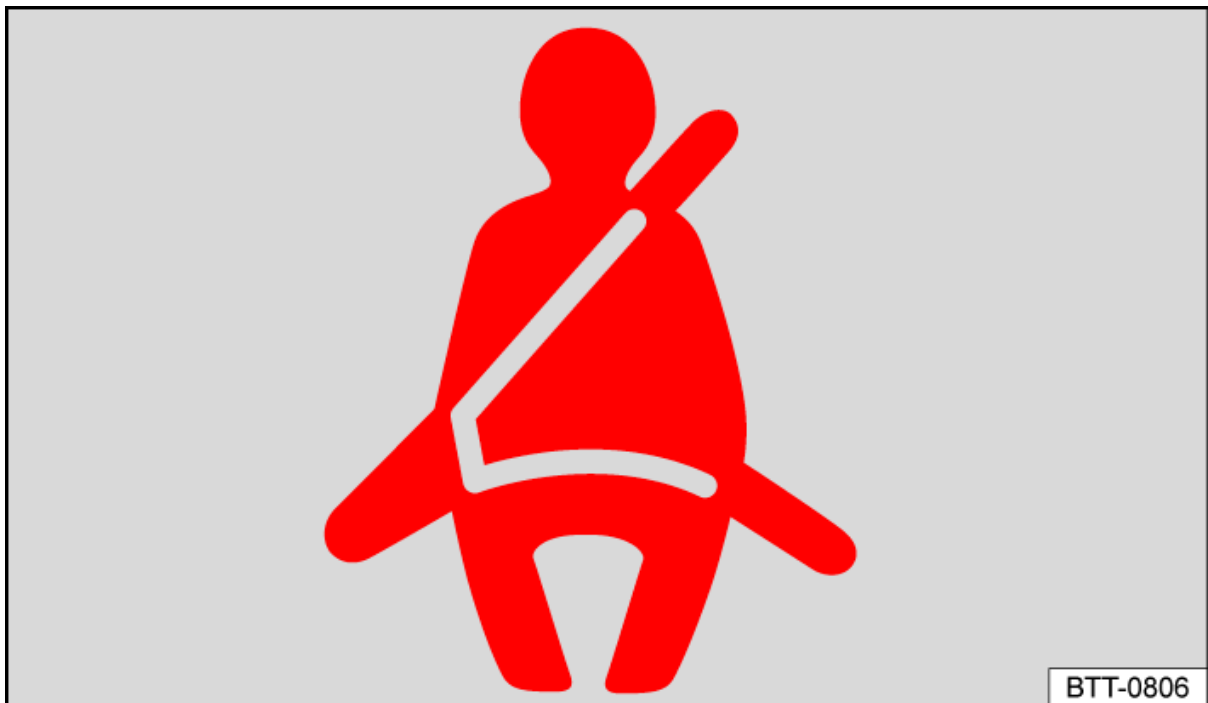
Fig. 1 On the instrument cluster display: warning lamp.
