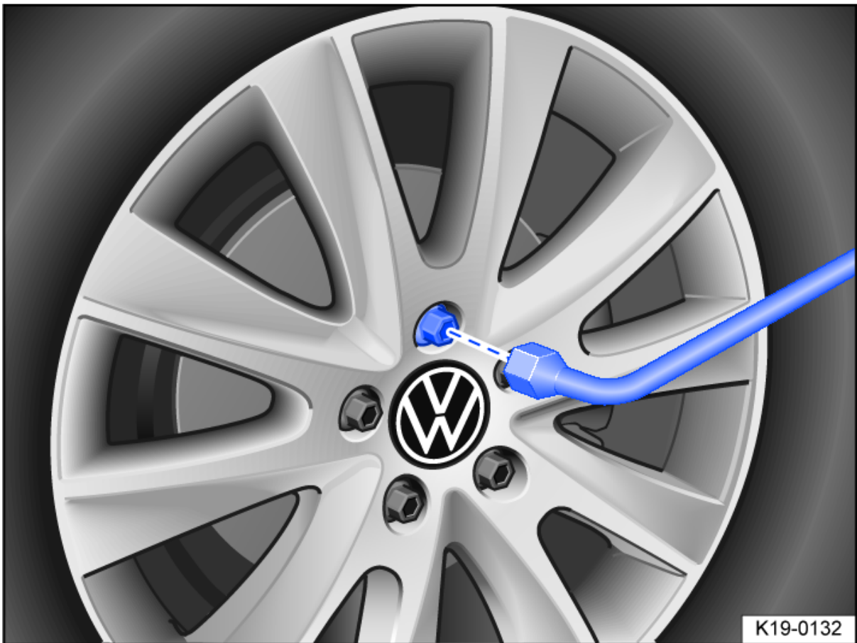
Fig. 1 Changing a wheel: removing the wheel bolts with the screwdriver handle.
