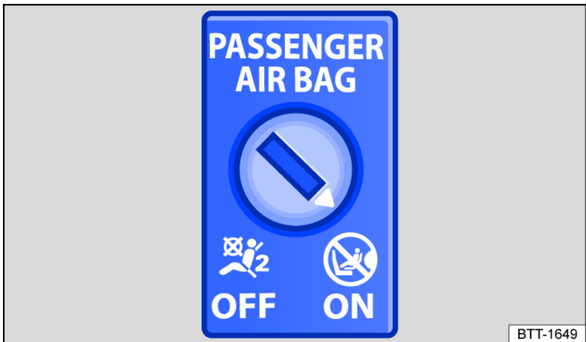
Fig. 1 In the dash panel on the front passenger side: key-operated switch for deactivating and activating the front airbag on the front passenger side
