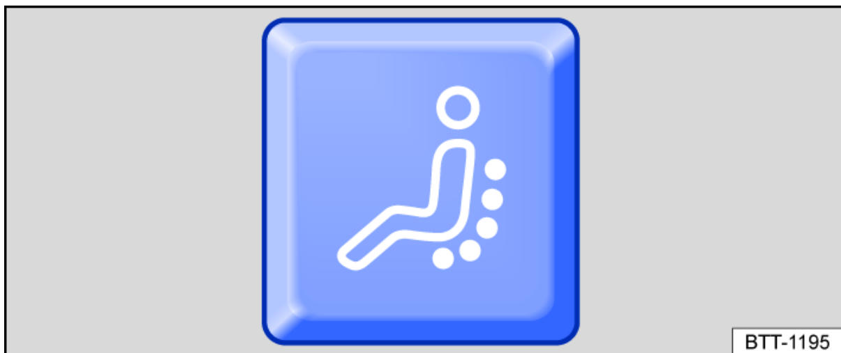
Fig. 1 In the lower area of the driver seat: button for massage function.
