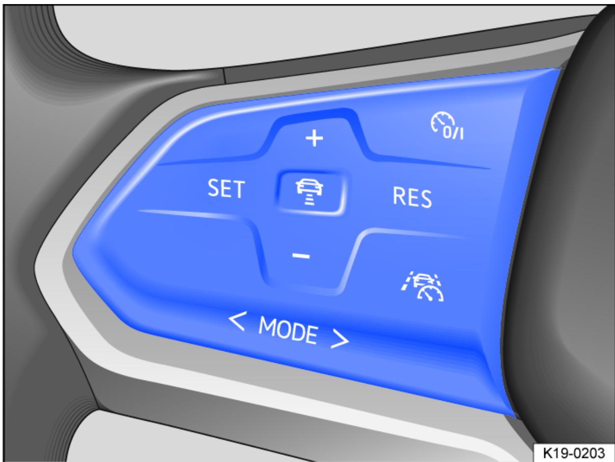
Fig. 1 Left-hand side of the multifunction steering wheel: buttons for operating the speed limiter.
