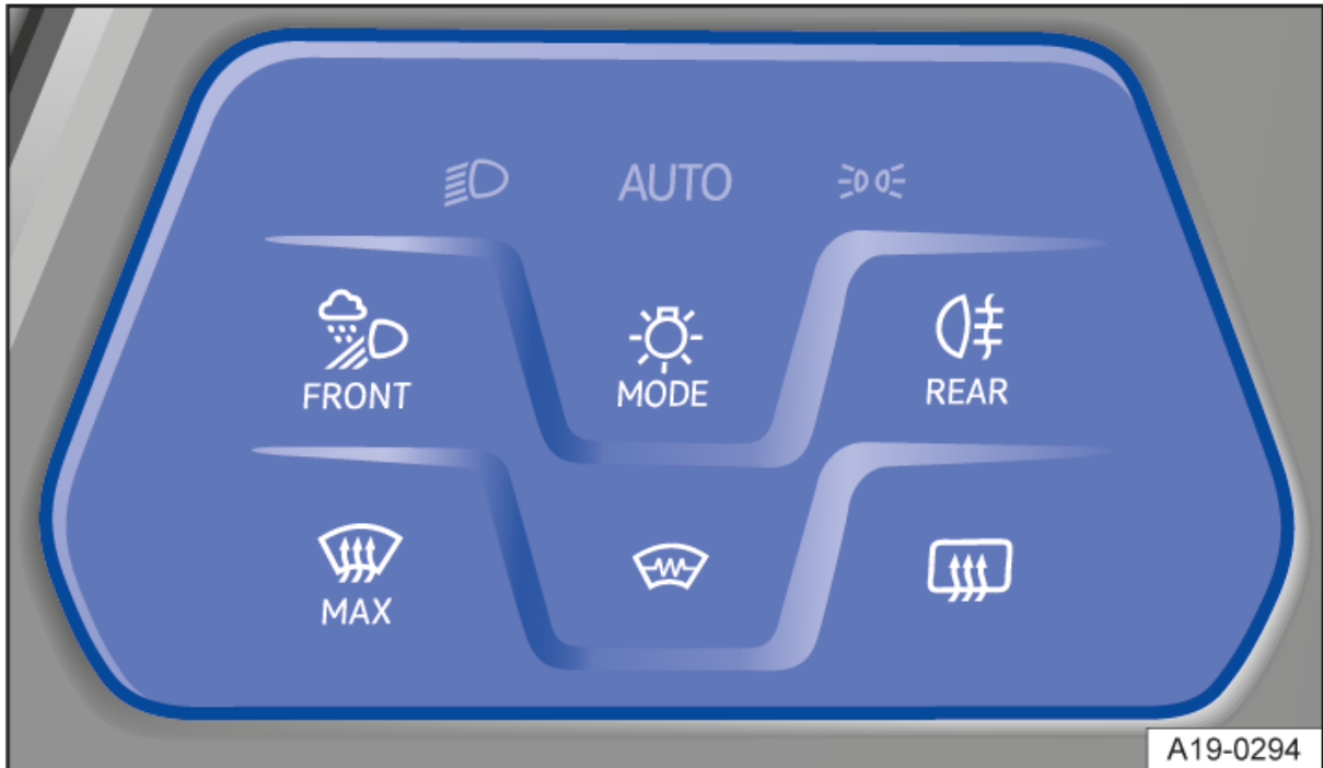
Fig. 1 Next to the steering wheel: control field for switching on the exterior lighting.
