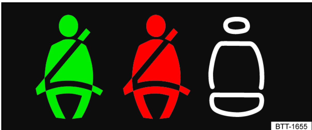
Fig. 2 On the instrument cluster display: seat belt status for the rear seats.
